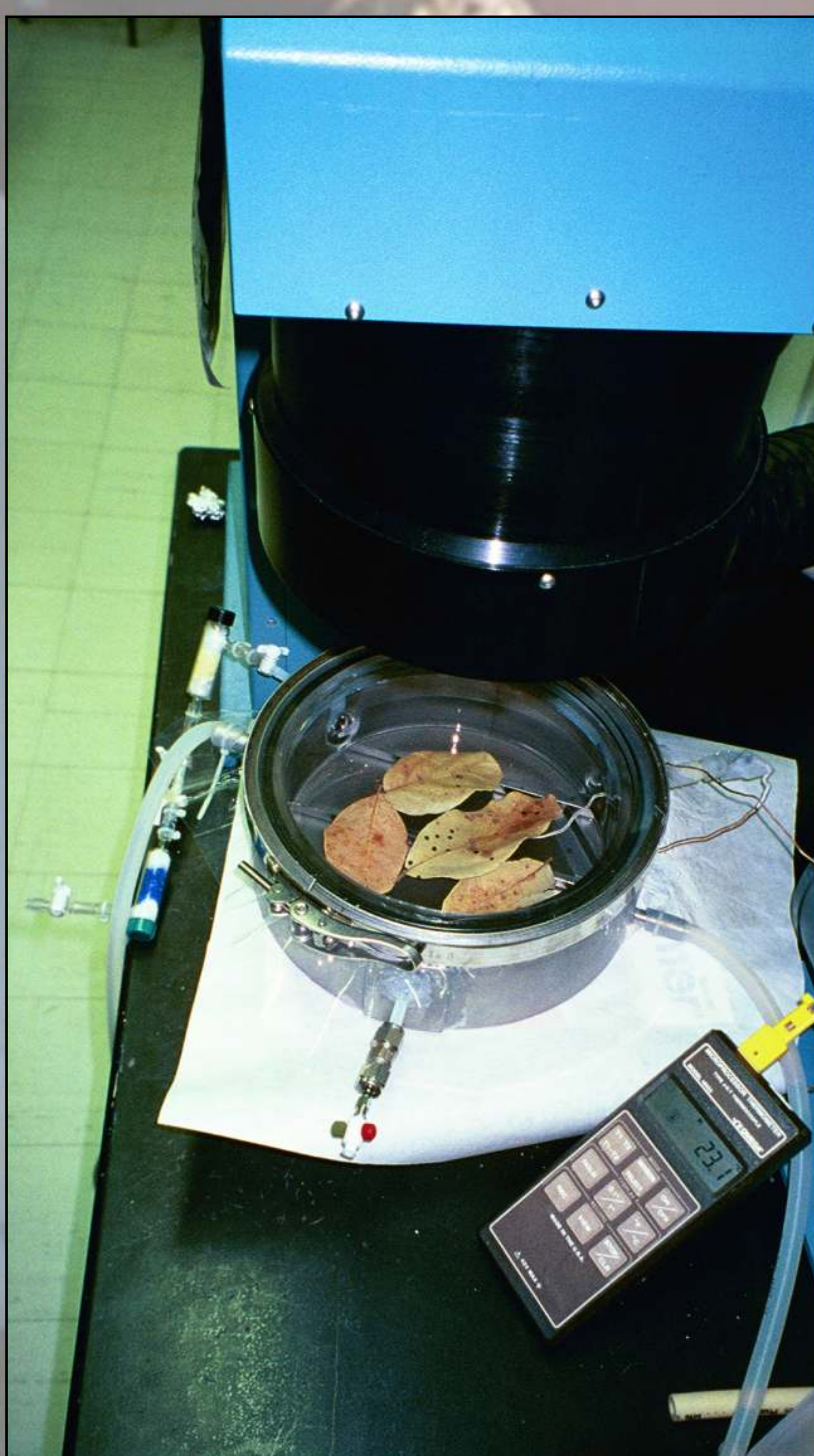
Figure 2. Apparatus used to investigate effects of light and temperature on plant litter production of NO x .
