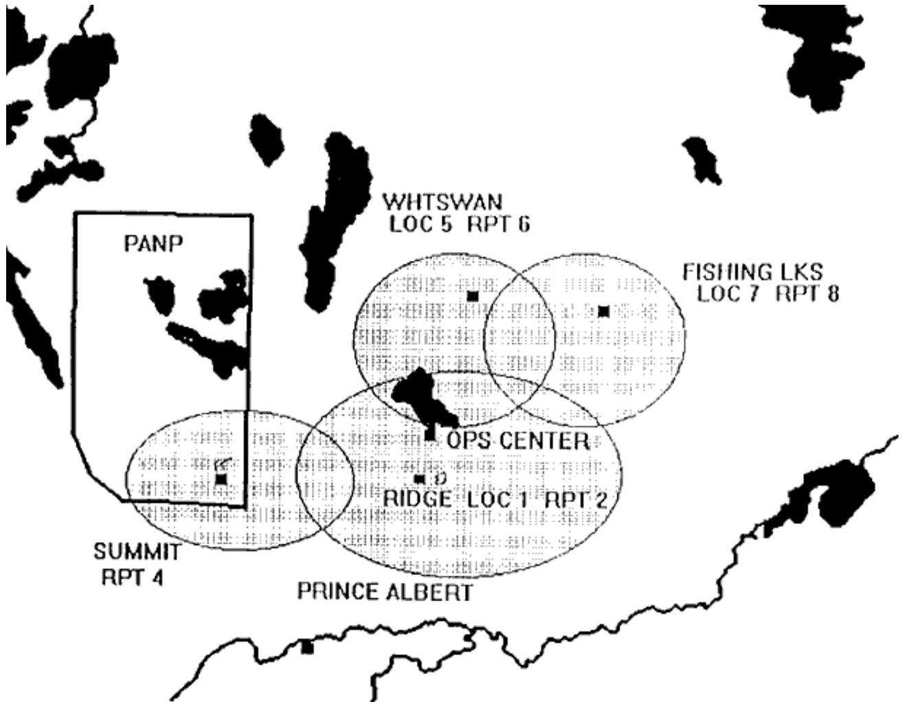
Figure 4.1.6.2 Ground radio net repeater coverage in SSA. Users should select channels denoted by RPT.
